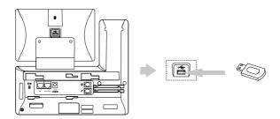
Note: The USB port (on the rear of the phone) can also be used to connect ZIP 450M Expansion Modules or a compatible USB headset.
