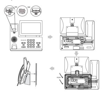
Note: The reversible tab has a lip which allows the handset to stay on-hook when the phone is mounted vertically.
