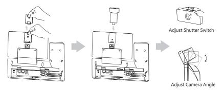
Note: The optional camera can only be connected to the USB port on the top of the phone.
